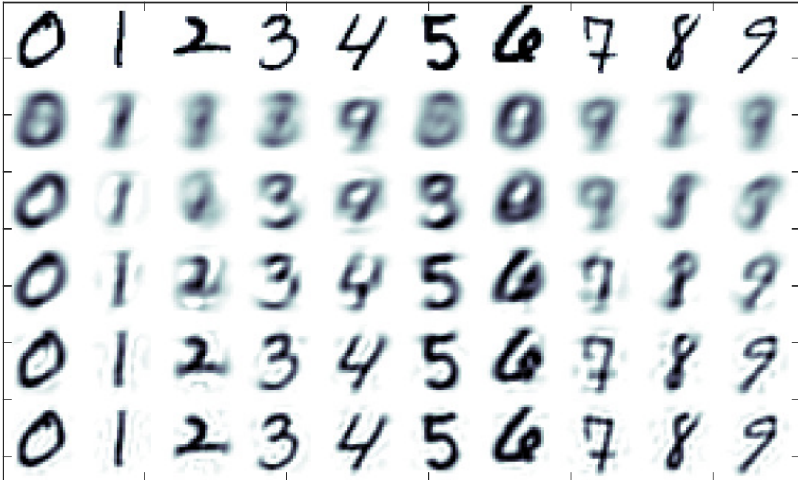
Fig. 3.12. Top row: 10 randomly chosen digits from the MNIST dataset. They are then reconstructed from n = 2, 5, 20, 50, 100 PCA components in the next 5 rows. We see that about 50 principal directions is enough to make a fairly good reconstruction of the images corresponding to a compression factor of about 16.
