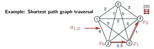
Find shortest path from starting node  $x_0 = 2$  to final node t = 5State Current node  $x_k = 4$ Actions next possible node:  $u_k \in \{1, 2, \dots, 5\}$ Dynamics Deterministic, known
