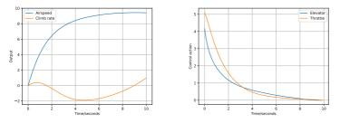
Left: airspeed and climb rate. Right: Elevator and throttle Why does the output adjust quickly but fail to get entirely to the goal  $y^*$ ?
